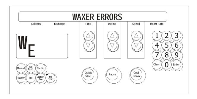
Upon entry into this test the letterw WE (waxer errors) will be in the profile window. This test allows you to see the current wax motor error conditions.
